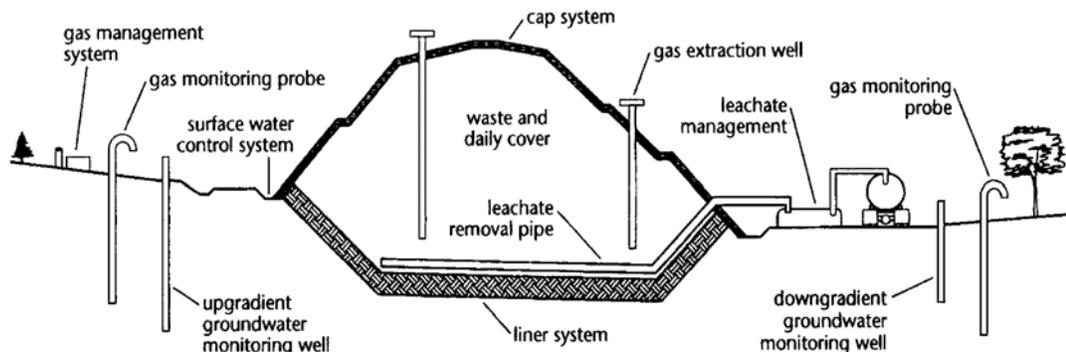
Note: the use of a tanker truck may not be practical as a method of leachate removal in areas of high rainfall and piping to a treatment facility is more appropriate.
