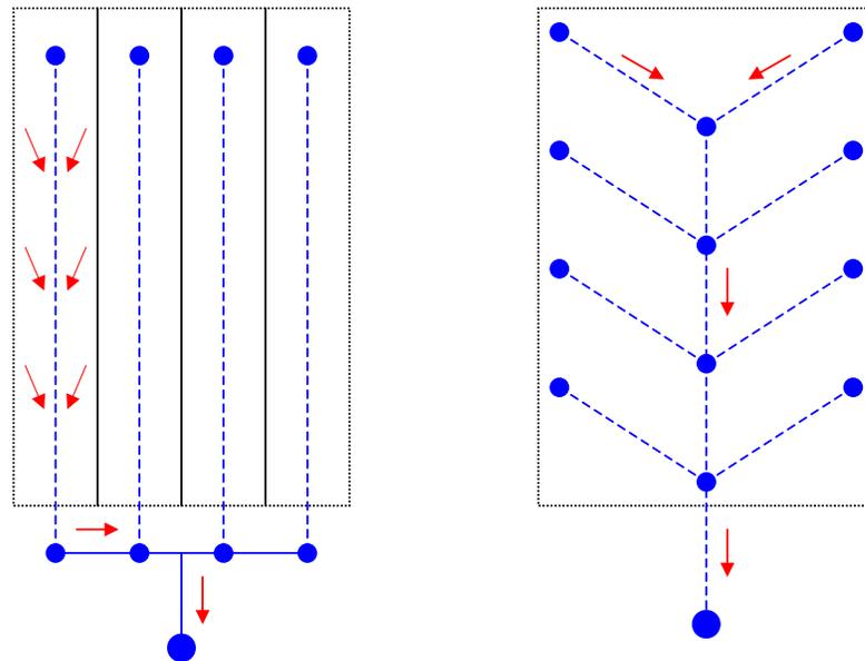
Figure 21. Typical Pipe Network for Leachate Collection
