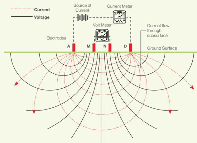
Figure 16.9 Equipotential and Current Lines for a Pair of Current Electrodes A and B
