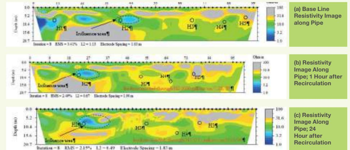
Figure 16.11 Resistivity Profiles Inside a Bioreactor Landfill after Leachate Recirculation (Ref: Manzur, 2012)
