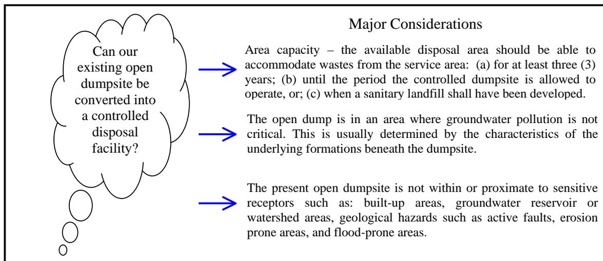
If the existing open dump does not meet most of these criteria, especially the groundwater pollution potential, it is not recommended for conversion into a controlled disposal site. Instead, a new site should be developed.
