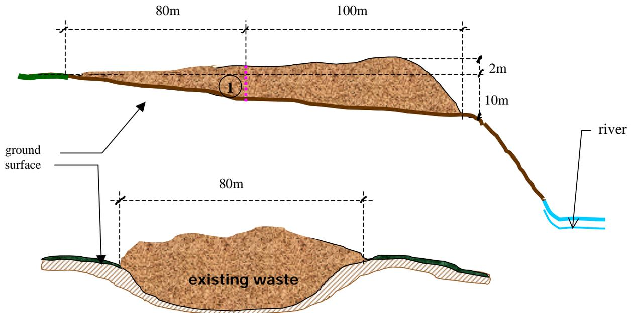
Figure 32. Approximate Profile and Cross-section of the Waste at the Site
