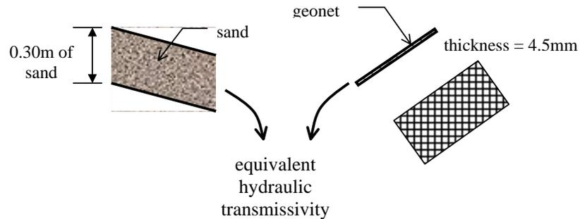
Figure 19. Geonet Compared With a Layer of Sand
