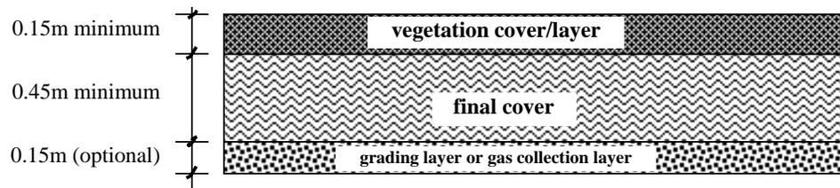
Figure 11. Recommended Final Soil Cover
