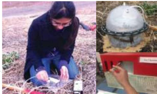
Figure 16.1 Flux Chamber Sampling and Determination of Concentration with Gas Chromatograph (Samir, S., 2014)
