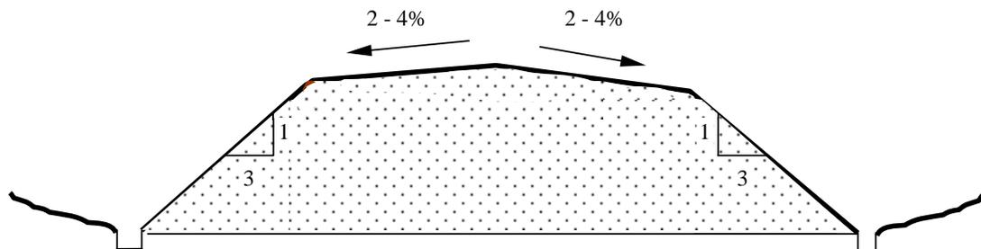
Figure 10. Grading of the Final Surface
