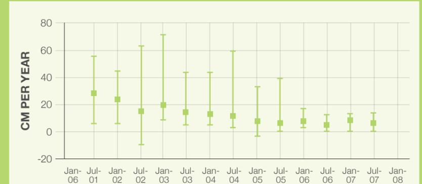
Figure 19.2 Settlement (average and range of 17 measurements points) on a 22 ha landfill since operation ended in 2000
