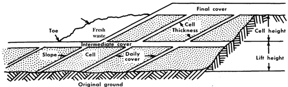
Figure 26. Cross-section of a Completed Landfill
