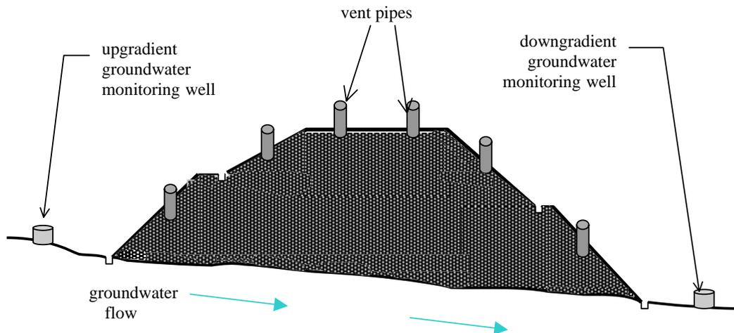
Figure 12. Vent Pipe and Monitoring Well Installation
