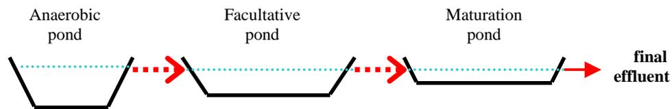
Figure 23. Layout of Waste Stabilization Ponds
