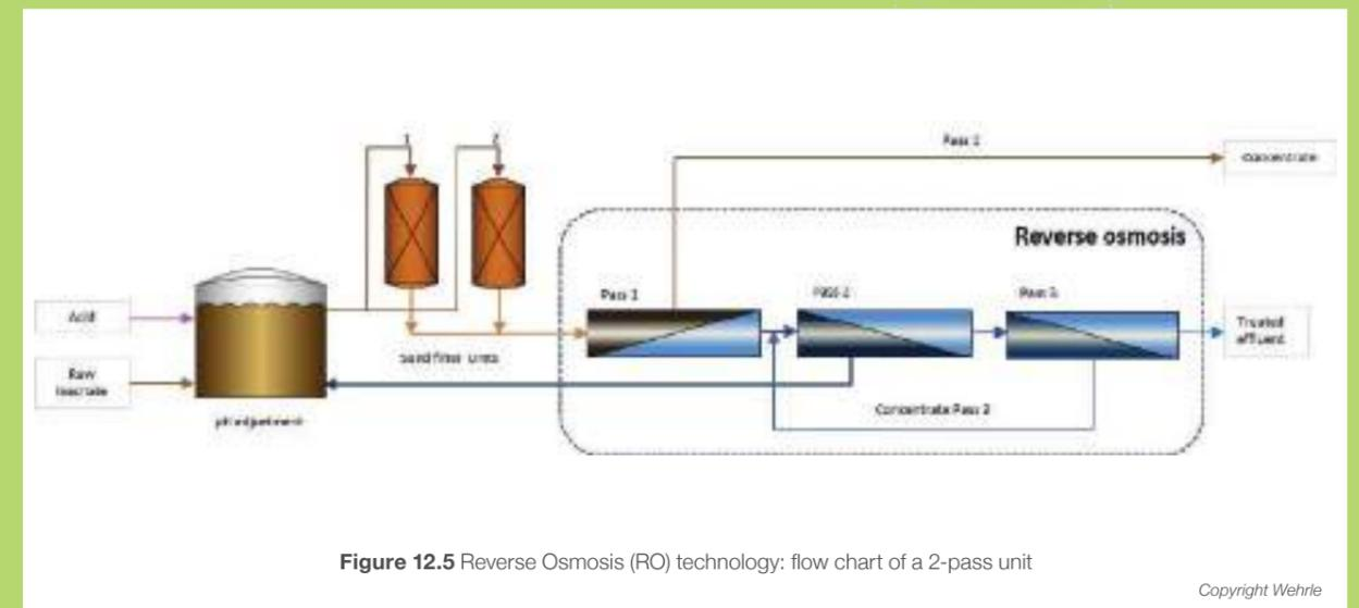
**Figure 12.5** Reverse Osmosis (RO) technology: flow chart of a 2-pass unit
