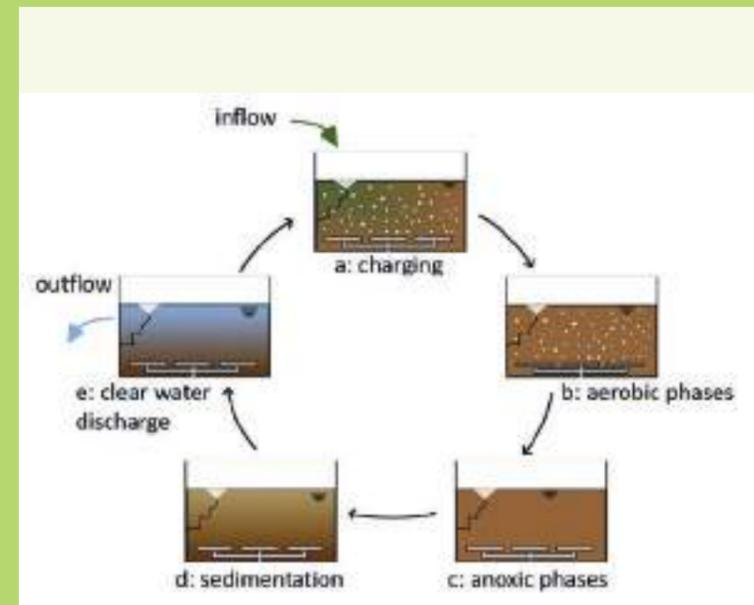
Figure 12.8 Biological “elimination” technologies: SBR process
