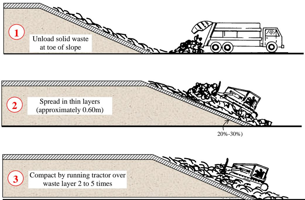
Figure 27. Waste Spreading and Compaction
