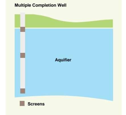
Figure 16.4 Multiple Grouped Ground Water Monitoring Well
