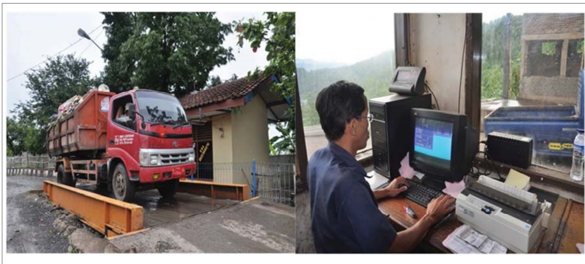
Figure 6 Measuring and recordkeeping incoming waste, (a) the waste vehicle truck pass weighbridge, and (b) weighbridge operator input necessary data for recordkeeping of incoming waste.
