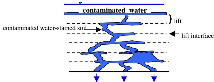
Figure 25. Liquid Flow Through Waste Cell Lifts
