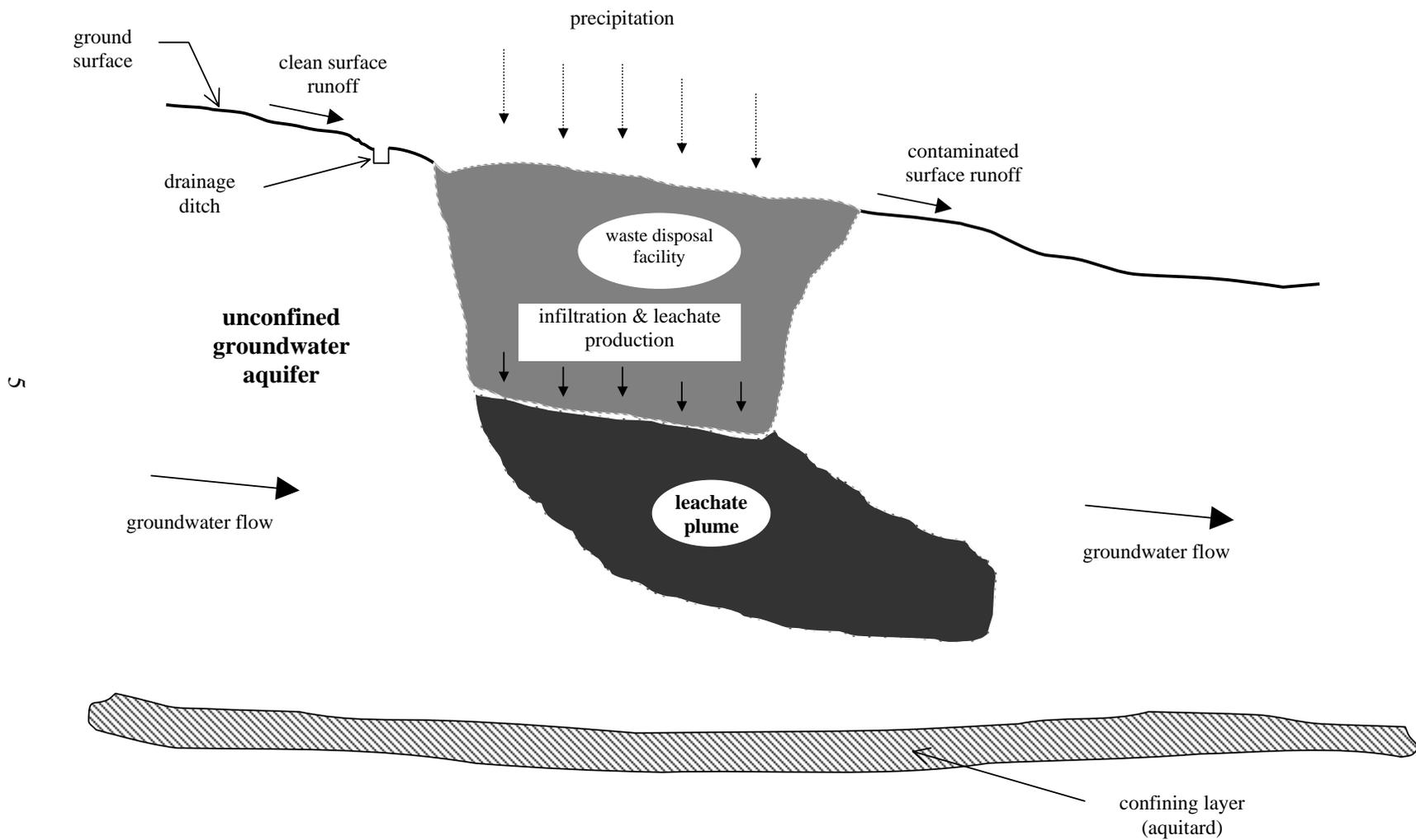
Figure 1. Water Pollution from a Waste Disposal Facility (over an unconfined aquifer)
