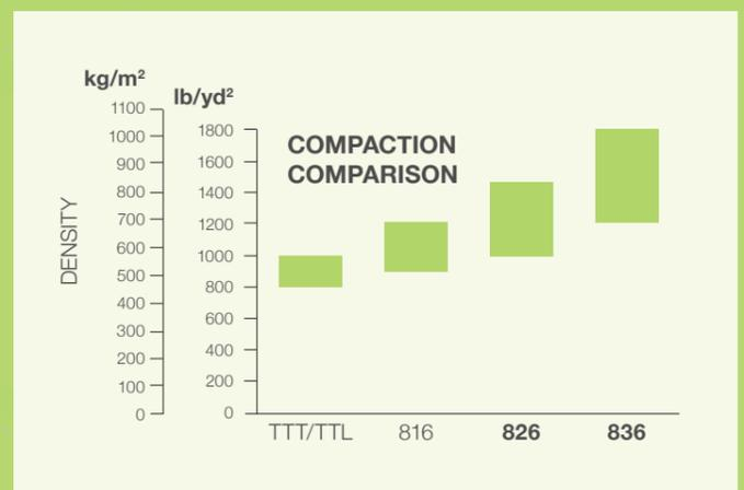
Figure 8.8 Compaction Performance Comparison – Track Type Dozers vs. Compactors
