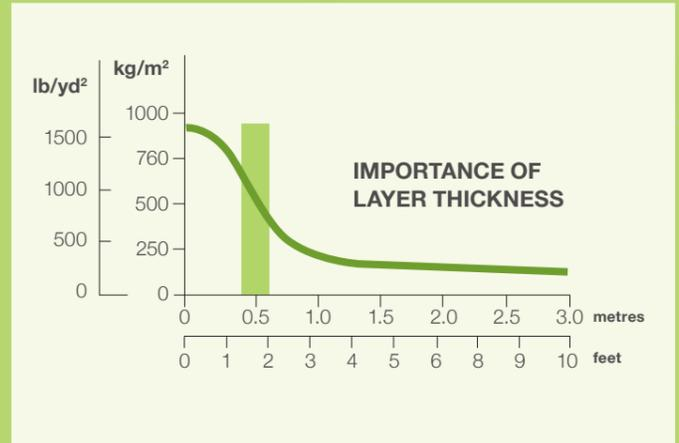
Figure 8.5 Optimum Compaction and Waste Layer Thickness
