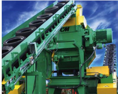
① - Primary/Chipping Shredder
