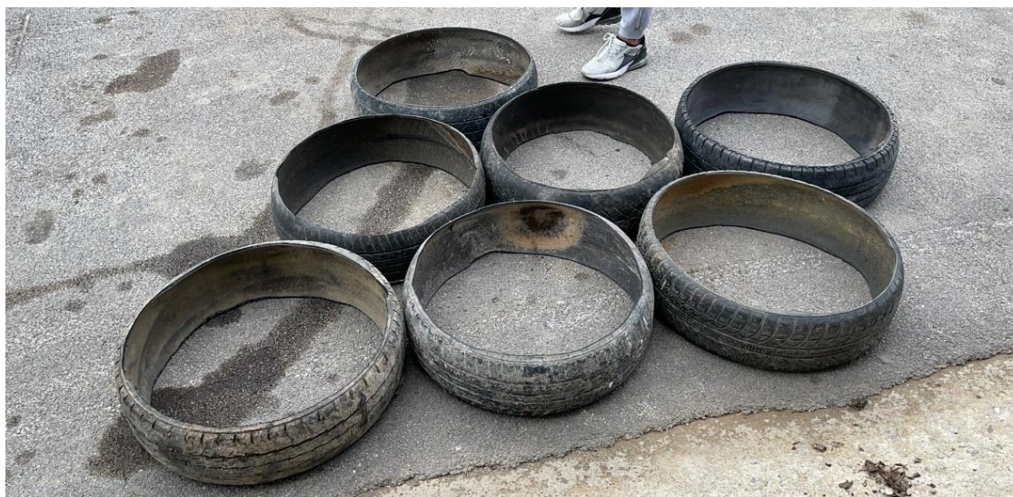
Figure 12: Geogrid from tyres (RWA, 2020)
