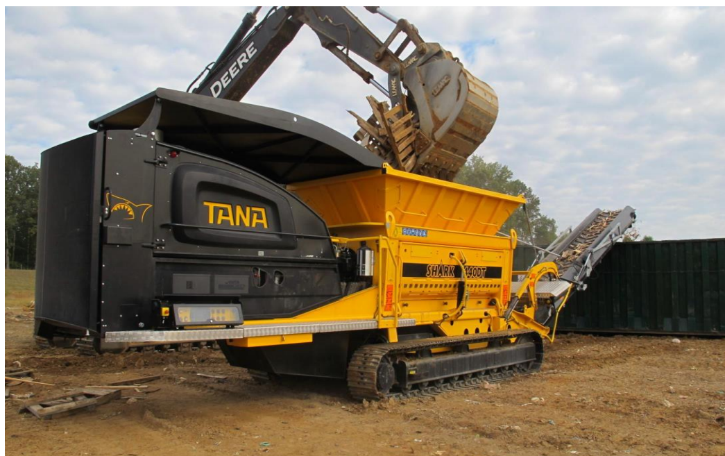
Figure 11: TANA Shark 440 Mobile shredder ( https://tana.fi/stories/tana-shredding-variety-of-materials/ )
