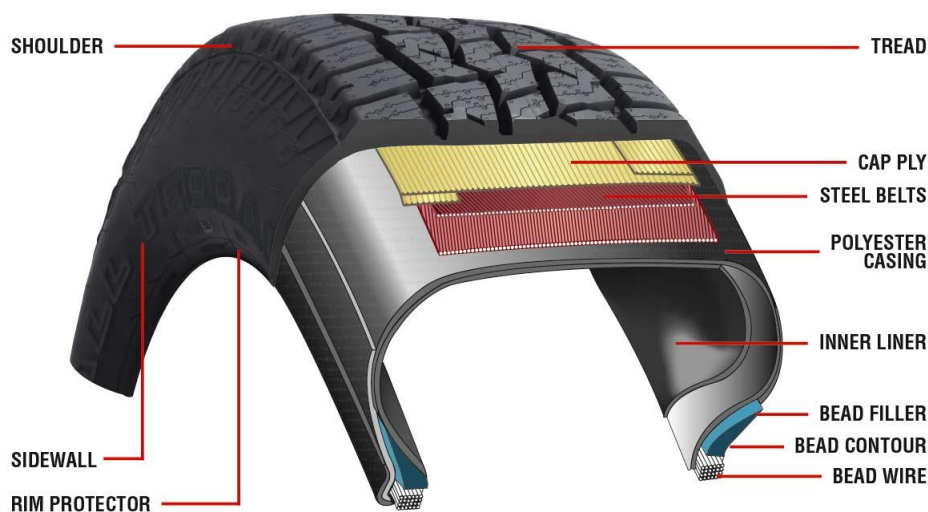
Figure 1: Construction of a typical tyre ( https://www.lesschwab.com/article/tire-faq.html )
