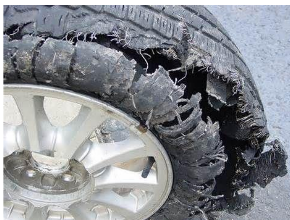
Figure 3: Steel wire strands from the tyre belt visibly protruding from the rubber tread in a “blow-out” tyre ( https://www.fastcompany.com/1788639/renewable-rubber-next-step-truly-oil-free-cars )
