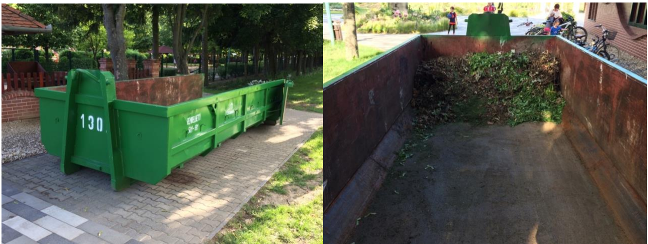
Figure 10: Example simple hook loader container as mobile green waste drop-off point = Szombathely, Hungary
