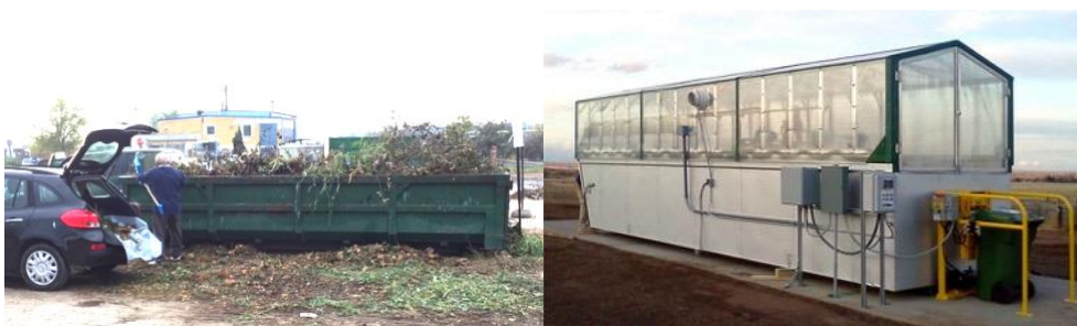
Figure 4: Example green waste drop-off containers and food waste pre-treatment container potentially suitable for the Kurina Facility
