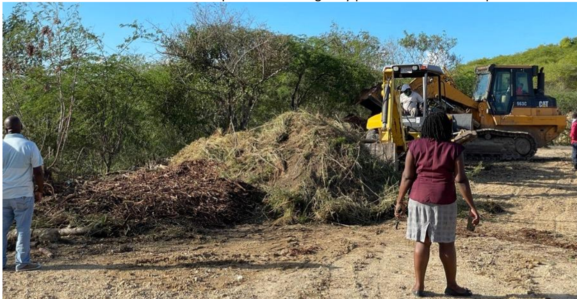
Machines can mix the materials as the pile is built and gently press it down into shape.
