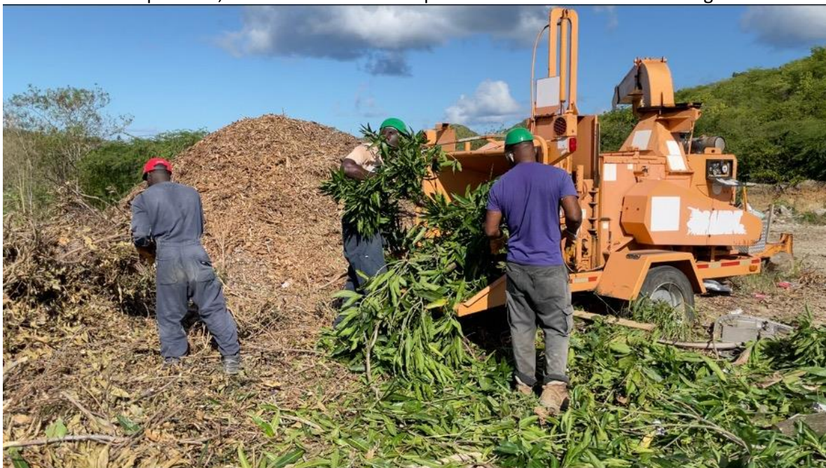
Once cleared of contaminants and, where required, chipped, the material is then layered into windrow compost piles, 20m long, 3.5m wide and up to 2m high.
